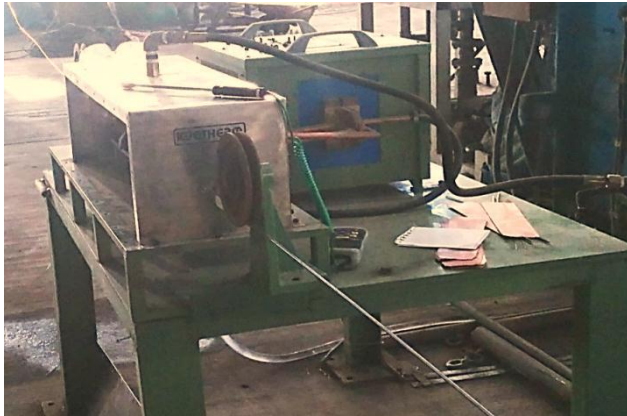
Figure 9 Induction Heating machine used for plant trial
